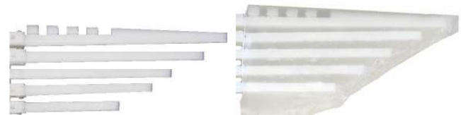
Fig. 13 Fin without and with flexible skin
