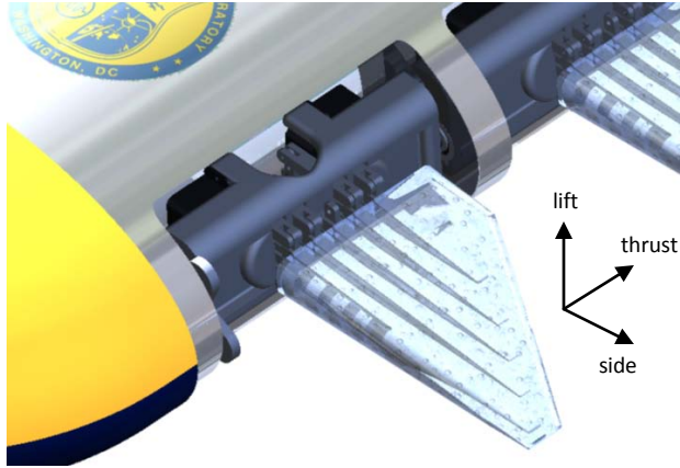
Fig. 1. Actively controlled curvature robotic pectoral fin mounted on custom designed UUV hull.
