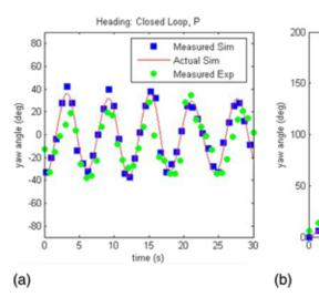
lated results is given. For a simple proportional control algorithm (Figure 12a), we see the results match well with a 30-40° amplitude and 6.5-s period. Dif-
