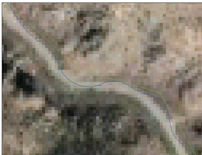
Figure 15. Results from the second flight through Goshen Canyon. Flight test results show the planned path (green) and the actual path (blue). The planned path was intentionally biased to the east, forcing the MAV to offset from its planned path of centering itself through the canyon.
